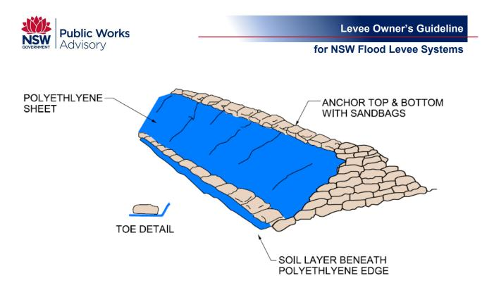
Figure 2 – Anchorage of polyethylene sheet with single row of sandbags
