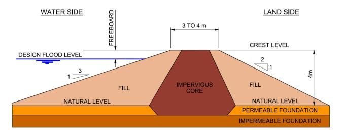
Figure 4-1 Typical NSW Earth Embankment Levee Design Cross-section
