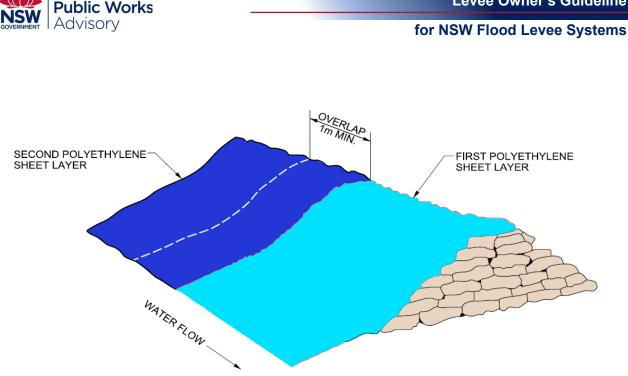
Figure 4 – Polyethylene sheet placement from downstream with overlap
