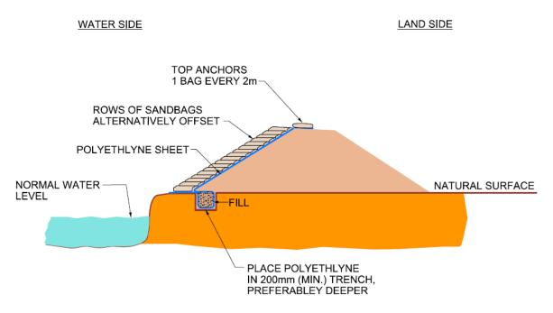
Figure 3 – Anchorage of polyethylene sheet in a trench (dry conditions)
