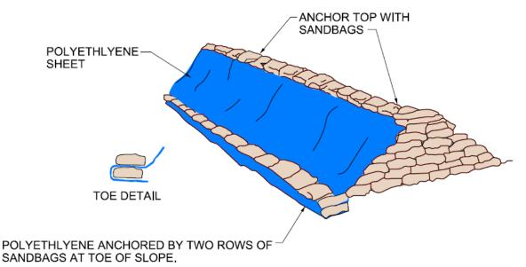
Figure 1 – Anchorage of polyethylene sheet with two rows of sandbags
