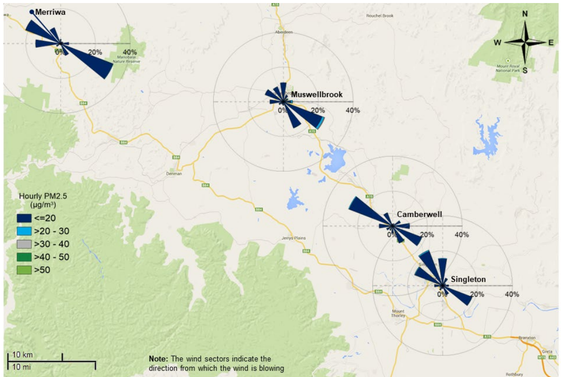
Figure 4 Hourly PM2.5 pollution rose map for the Upper Hunter region for autumn 2023
