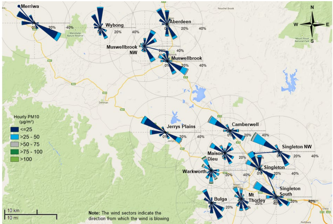
Figure 3 Hourly PM10 pollution rose map for the Upper Hunter region for autumn 2023
